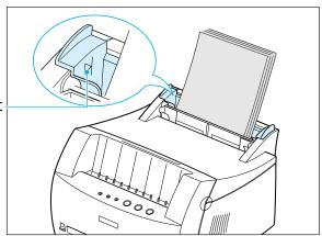
5 Adjust the paper guides to the width of the paper stack.
